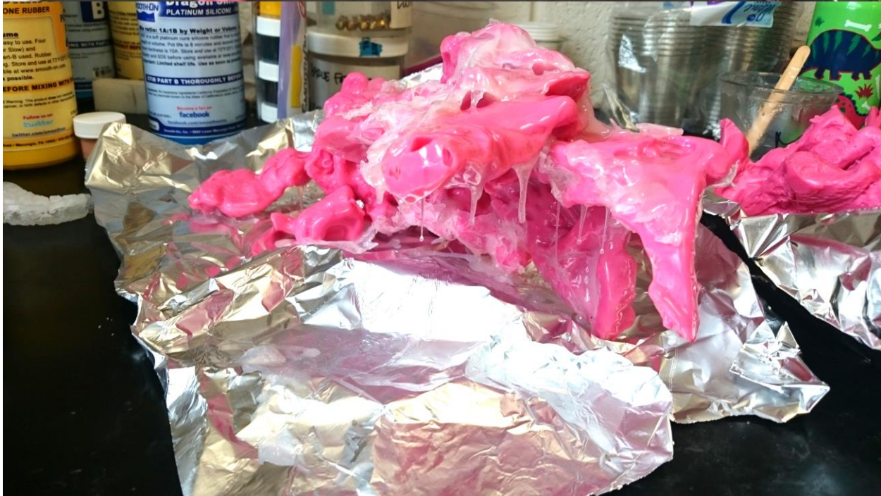
The pink wax injection castings demolded and joined with others to elaborate more complex structures. The Dragon Skin silicon rubber was then layered in different colors, one at the time. Every layer took approximately 30 minutes to finish.
