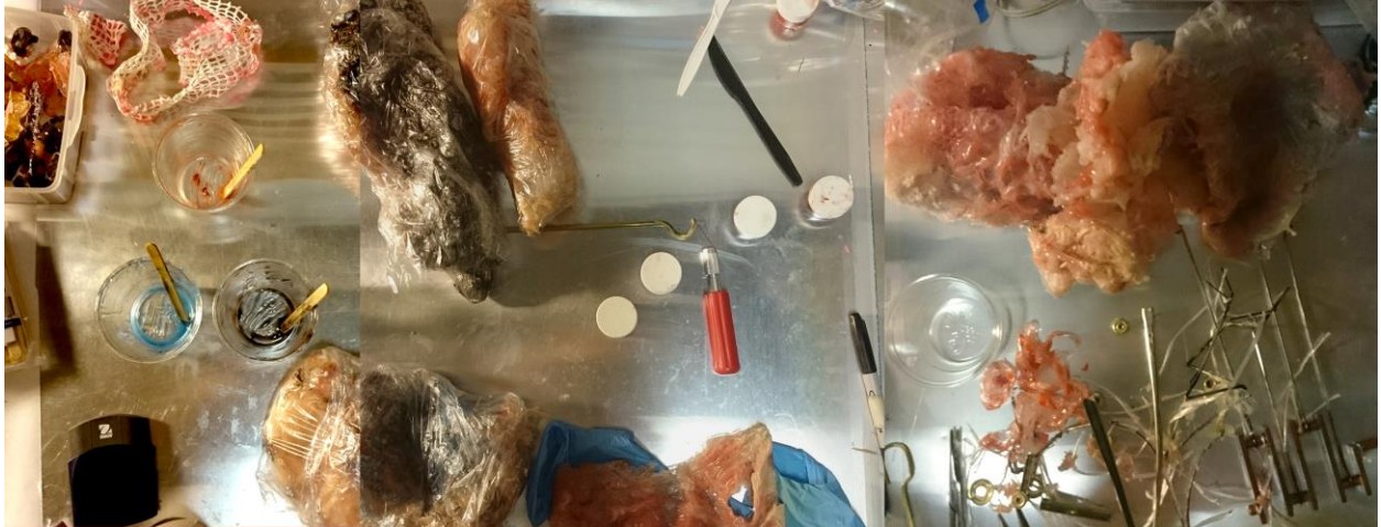
Birds-eye view of the work bench. Silicon layers were applied with the help of plastic wrap that allowed its own texture and made it easier to demold and reuse. The Dragon Skin is a two-part mix that must be measured precisely, the color has to be applied in the initial mix.
