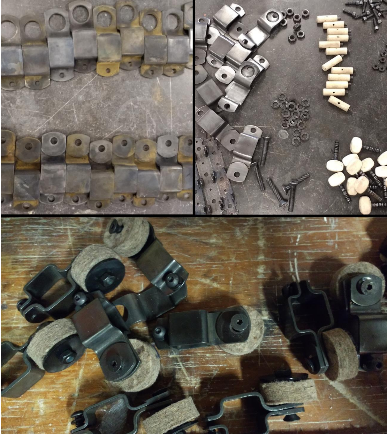
Details on the process and finish of the hardware. The clamps were refinished to be able to hold cymbal felts to dampen the vibration. All the metallic pieces were darkened with a gun blue patina sealed with paste wax.
