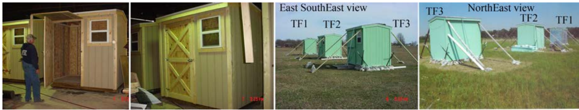
Fig. 2.2 Thermadapt™ Full Scale Test Facilities in the Fabrication Shop and on the Outdoor Test Range: Fabrication, Erection and Operation
