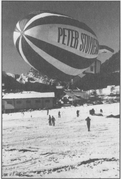
Figure 1. Thermal Airship, Thunder and Cold Balloons AS-100. (Courtesy The Association of Airship and Balloon Constructors)
