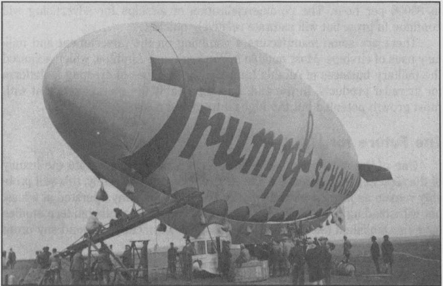
Figure 5. Semi-Rigid Airship—1930's Parseval-Natz PN29. (Courtesy The Association of Airship and Balloon Constructors)
