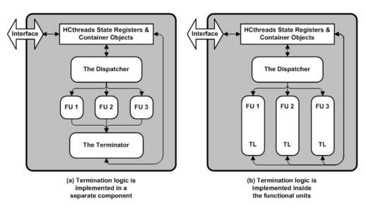
Figure 5.1. HCthreads internals assuming three functional units
