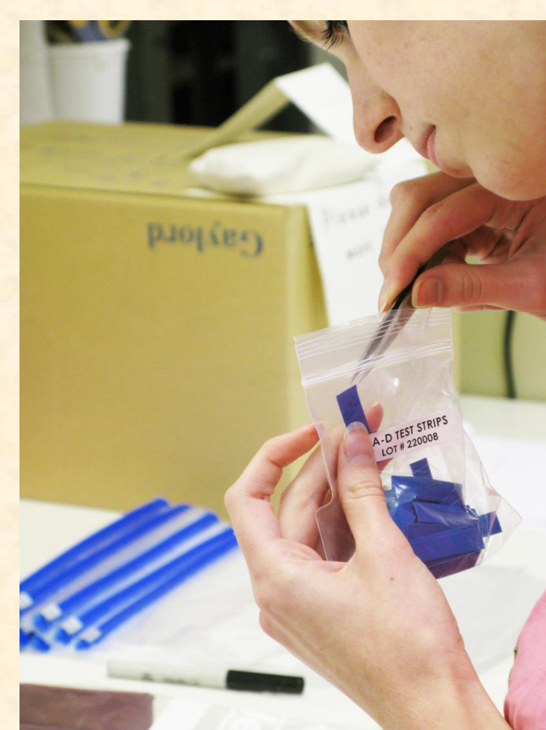
Reference pencil showing scale of 0 to 3, with 3 meaning extensive off-gassing. A-D strips were removed from storage bag with tweezers.
