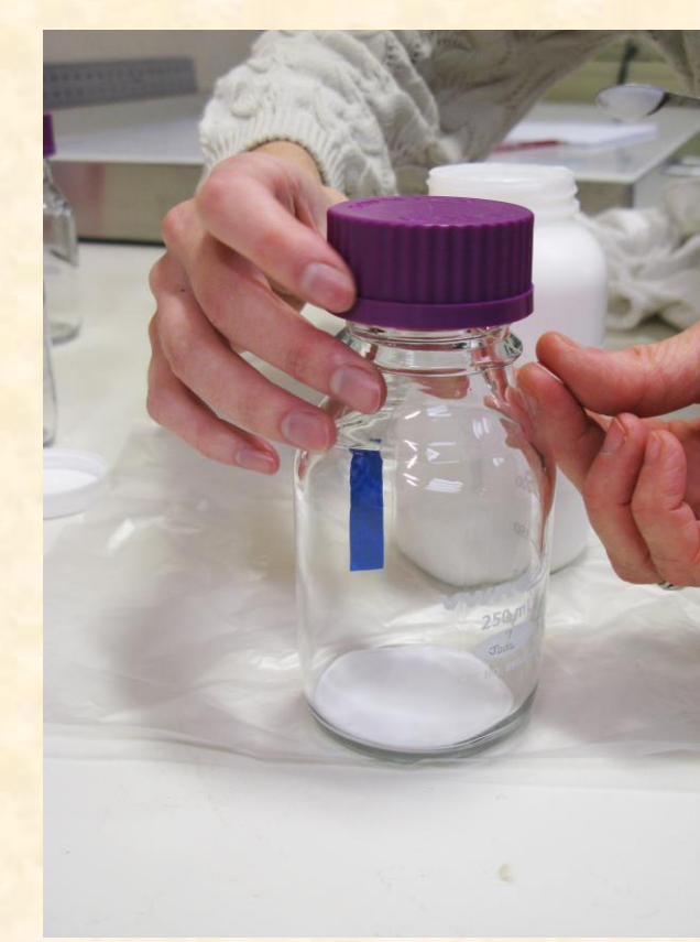
Components were tested individually in glass jars. Adhesives were measured out for consistency in each jar, A-D strip suspended by linen thread over adhesive, A-D strips checked at periodic intervals in order to track changes.
