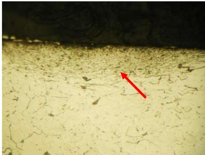
Photo 13. Sample 4-P. Microstructure at the surface of the hole, near mid-thickness of plate, showing a semi-circular zone of grain deformation and unresolved microstructure (arrow). (~500 X).
