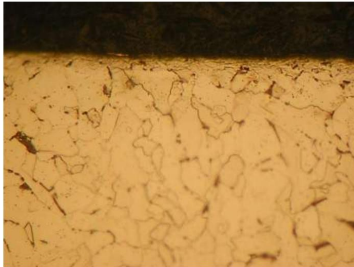
Photo 5. Sample 9-U. Microstructure, showing shallow depth of grain deformation at the surface of the hole, shown at top. (~500X)
