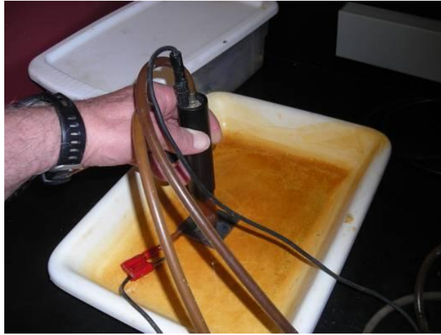
Figure 21. Electrolytical Polishing Tip Working on the Surface of Specimen
