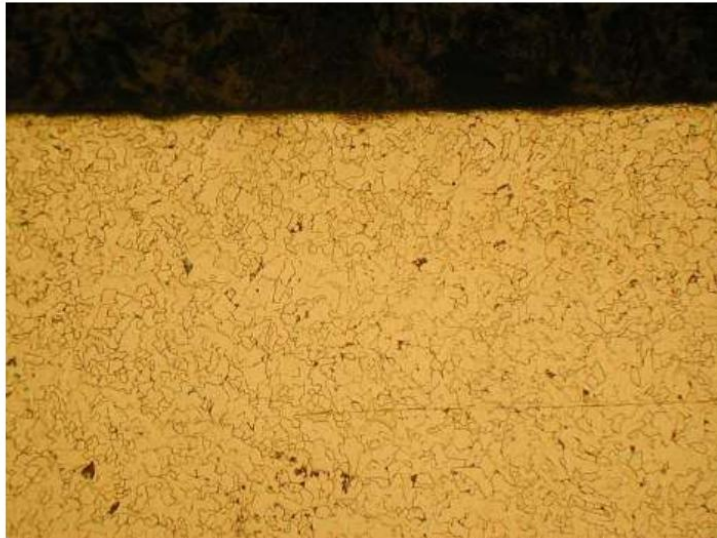
Photo 6. Sample 10-D. Base metal microstructure. Surface of the hole is at top. (~100X)
