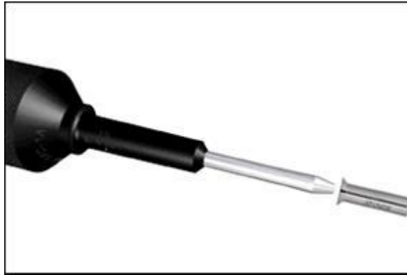
Figure 11. Cold Expansion Process. Pre-Lubricated Split Sleeve, Mandrel, and Hydraulic Puller (Fatigue Technology 2011)
