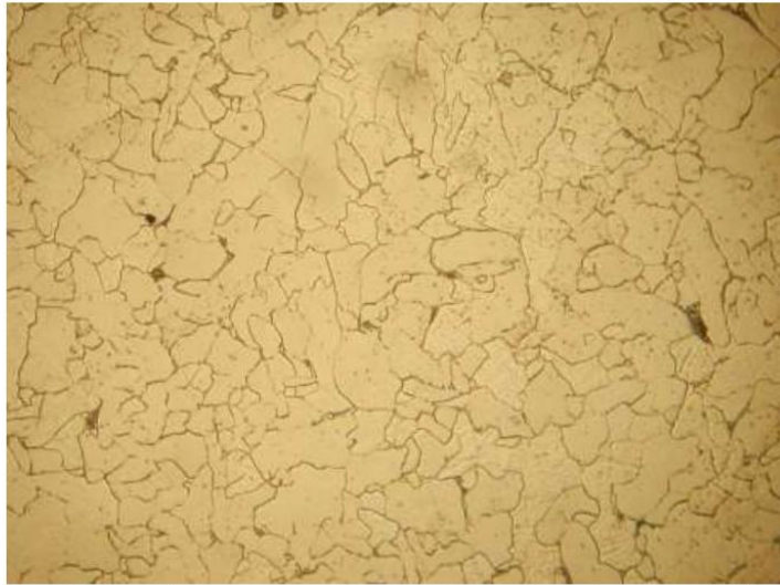
Photo 3. Sample 4-P. Microstructure of base metal away from the hole, exhibiting a ferrite matrix with dispersed pearlite colonies. (~500x)
