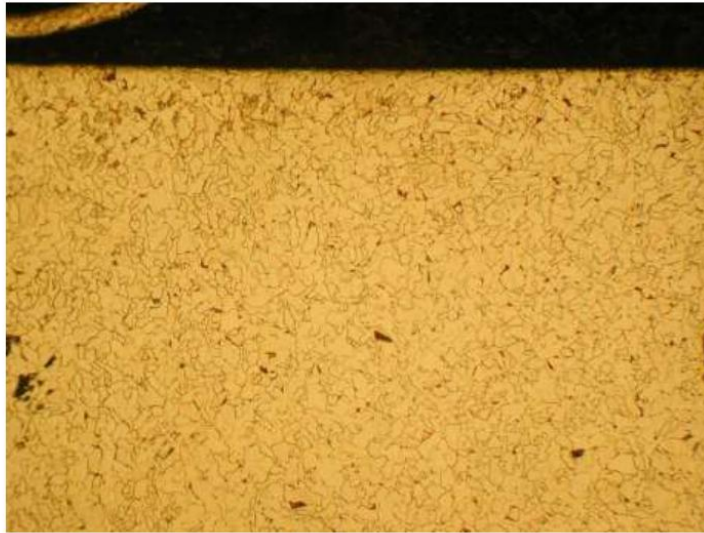
Photo 4. Sample 9-U. Microstructure of base metal. Hole bore surface is edge at top of photo. (~100X)
