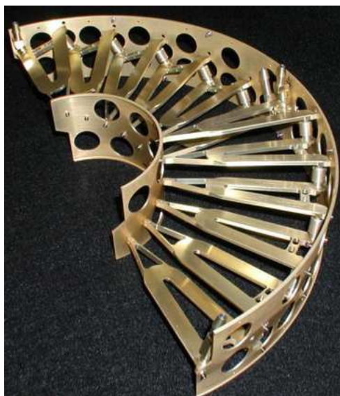
Figure 13: One half disk of the supporting structure of the FPix, showing the tilted blades [5].
