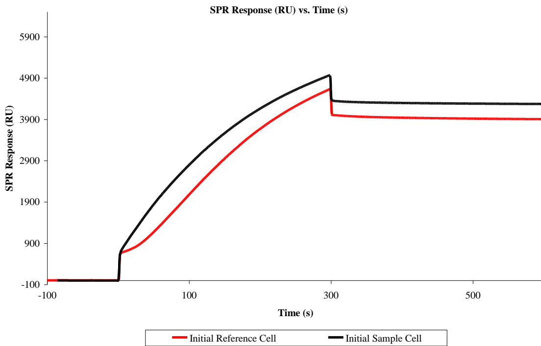
Figure 4.16: SPR sensorgrams of initial reference cell and sample cell F_1 -ATPase-His injection.
