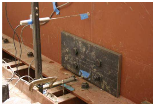
Figure 16. Retrofit measure 6: (a) 457-mm (18-in. long) backing plate on exterior side of web; (b) Maximum principal stress contours on the exterior side of web with the back plate removed from view; arrows point to point of highest maximum principal stress along HSS Paths 1 and 2. Cracks modeled using XFEM and
