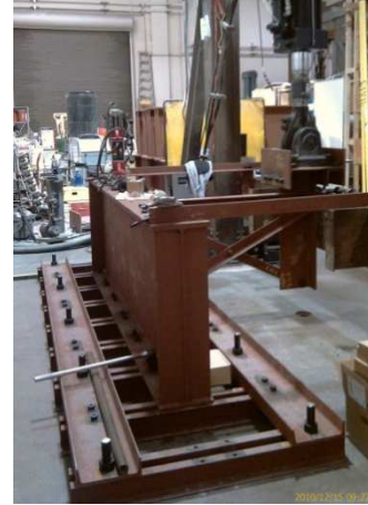
Figure 2. View of fascia side of girder specimen
