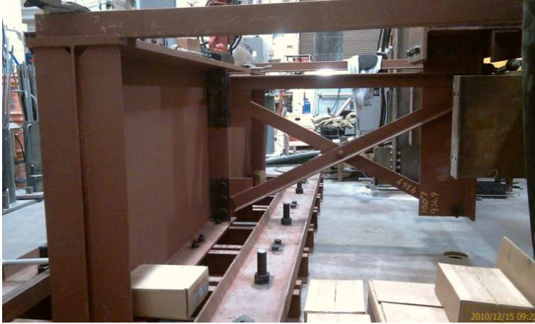
Figure 1. View of girder specimen
