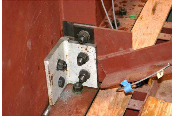
Figure 15. Retrofit measure 6: (a) Schematic of retrofit 6 (interior view); (b) Maximum principal stress contours in the web gap region with the angles removed from view; arrows point to point of highest maximum principal stress along HSS Paths 1 and 2. Cracks were modeled with XFEM and contour integrals. (c) Photograph of interior side of girder with stiffener-to-web angle and backing plate retrofit.
